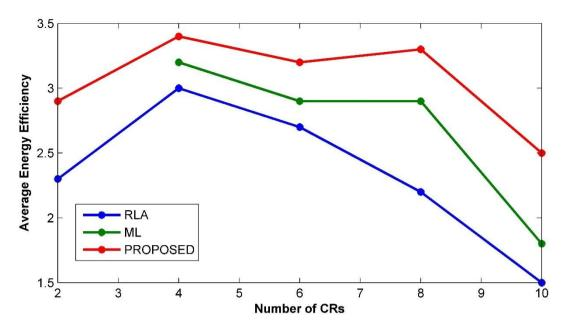
Figure 3: Performance analysis of average energy efficiency using RLA, ML and proposed techniques with different number of CRs. Here we observe that the average energy efficiency of proposed is better than RLA, ML.
