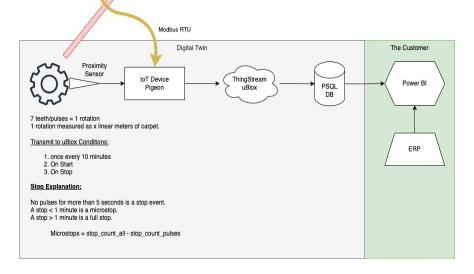
In the above machine the ELECTRIC METER collects the power consumed and the rotor sensor connected with a proximity sensor, collects the length of the manufactured carpet area, and correlates it with the power consumed.
