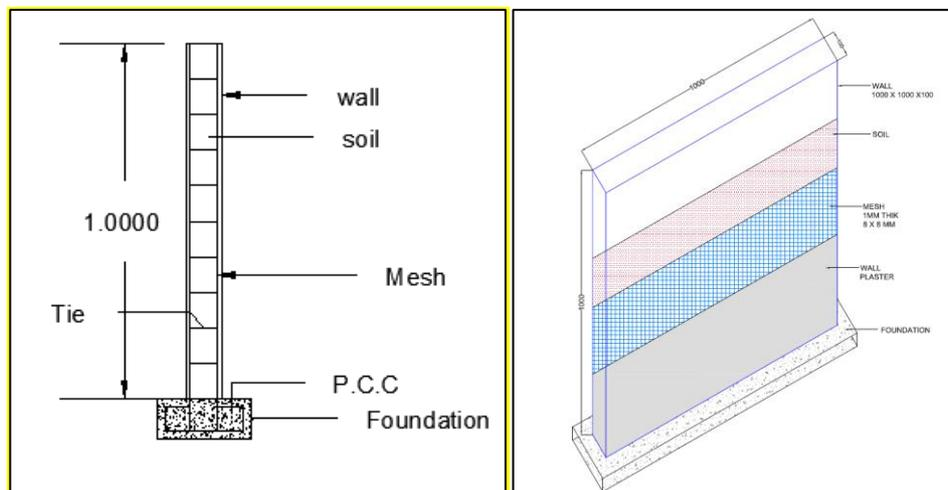
(a) Cross section of wall panel (b) Different layers of wall panels
