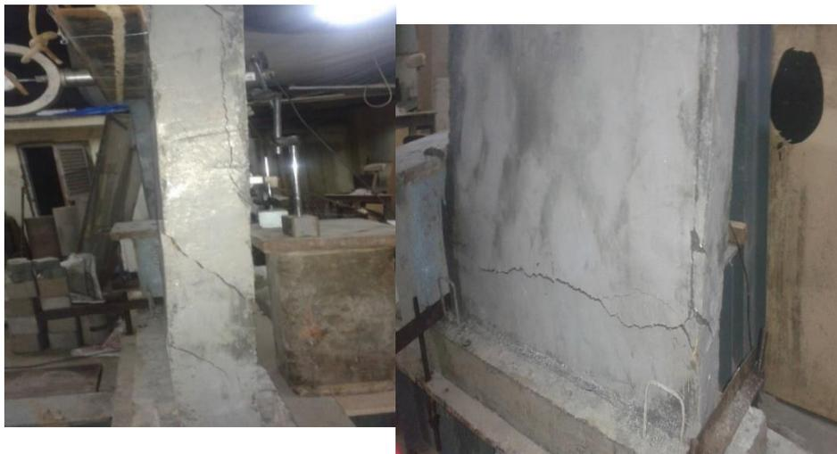
**Fig. 7 Initiation of cracks in the wall at bottom**
