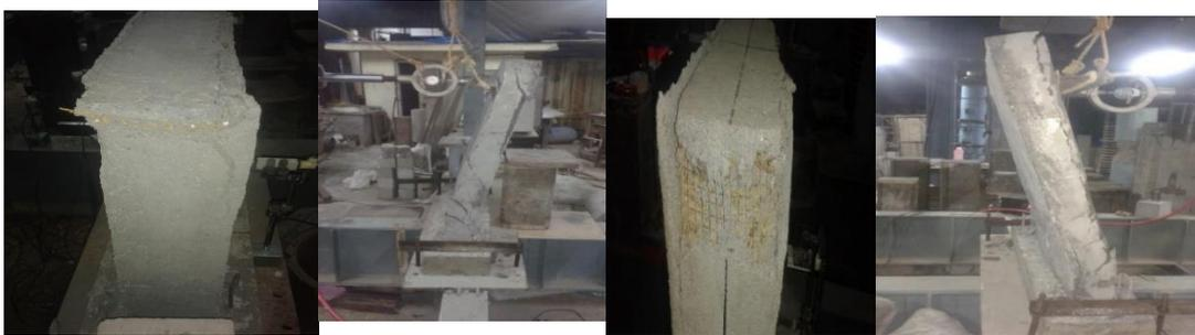
**Fig. 8 Final failure of wall panels at maximum load**
