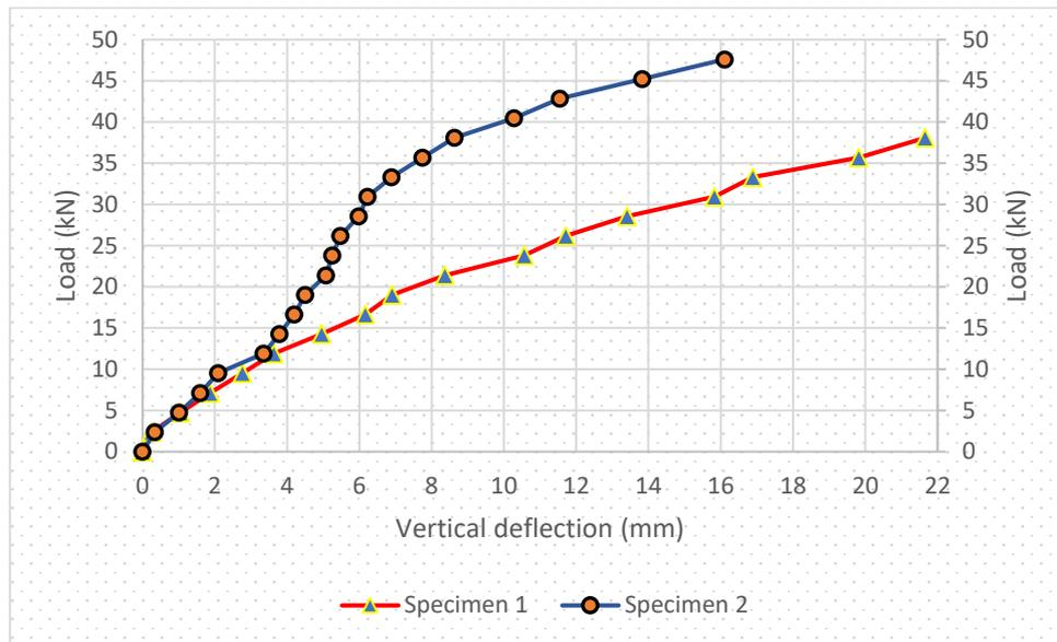
**Fig. 5 Load versus Deflection for Axial Load Test**
