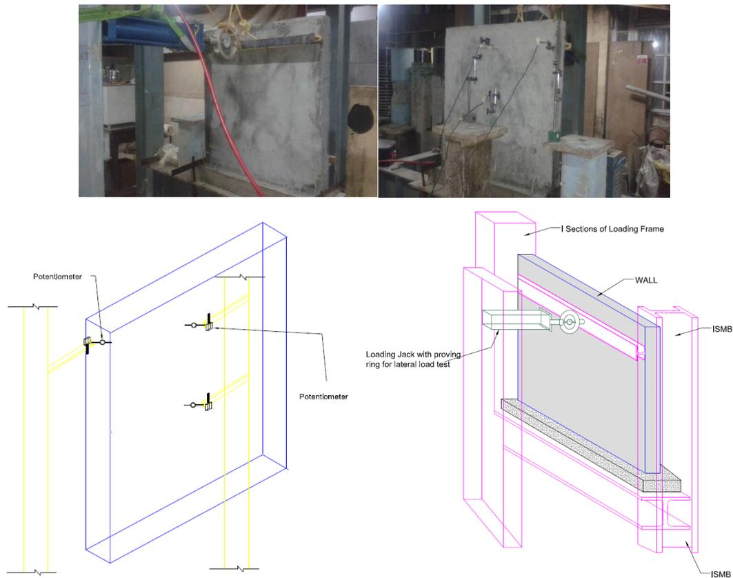
**Fig. 4 Assembly setup for lateral load test showing loading arrangement and placement of linear potentiometer**
