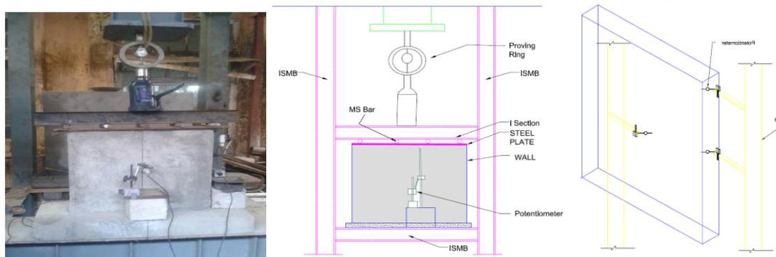
**Fig. 3 Assembly setup for axial load test showing loading arrangement and placement of linear potentiometer**
