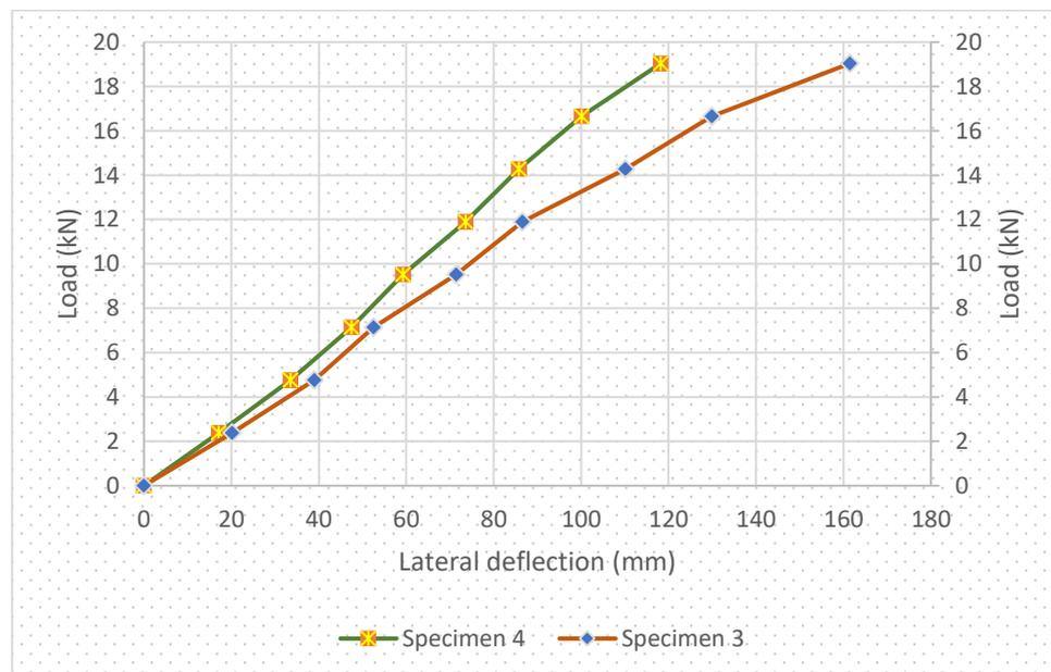
**Fig. 6 Load versus Deflection for Lateral Load Test**
