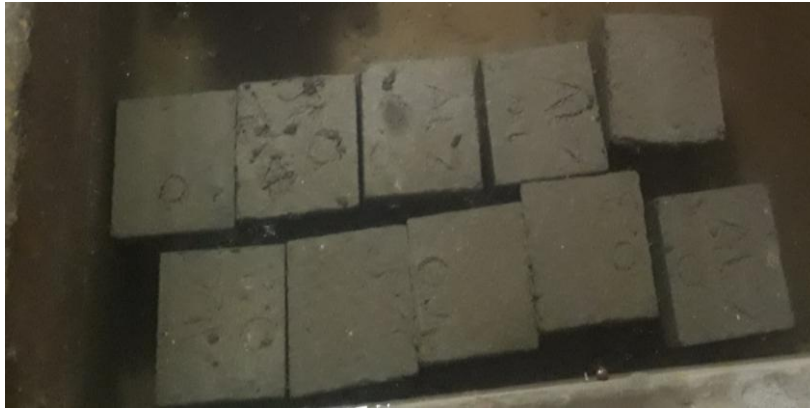
Fig8. Test Setup for Water Absorption
