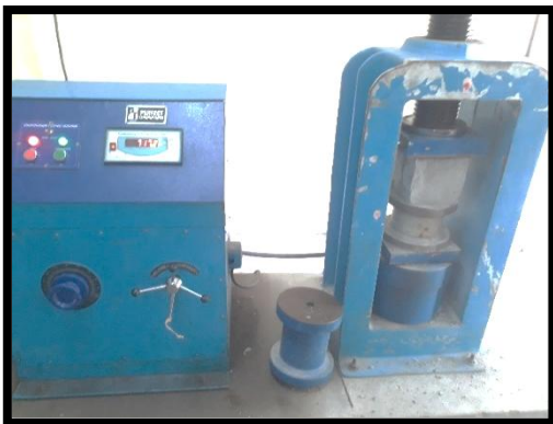
Fig 6. Test setup for cube specimen
