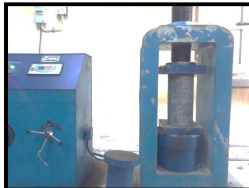
Fig 7. Test setup for cylinder specimen
