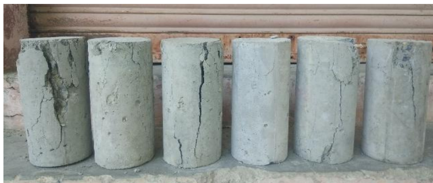
Figure 11. Failure Modes of Cylinder Specimen Under Compression Testing
