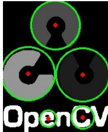
Fig. 2. Circle Detection using Hough Circle Method
