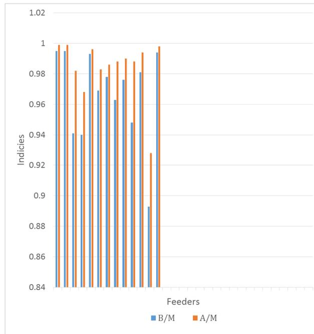
Figure 4.1: Operational availability of test bed feeders before and after monitoring
