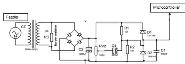
Figure 2: Signal sensing circuit for SACq
