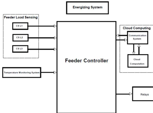
Figure 6: Overall block diagram for the monitoring and fault detection system
