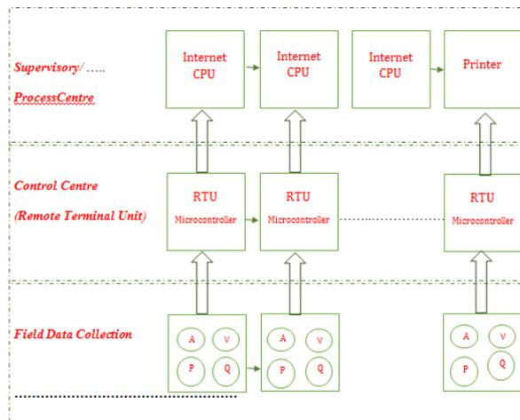
Figure 5: General layout design of monitoring and fault detection system in Medium Voltage Networks
