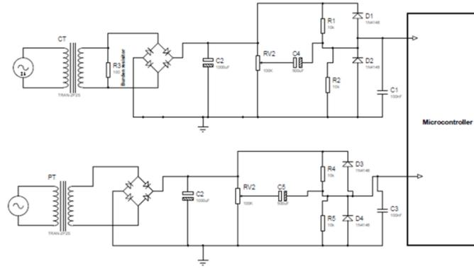
Figure 7: Current and Voltage measurement circuit
