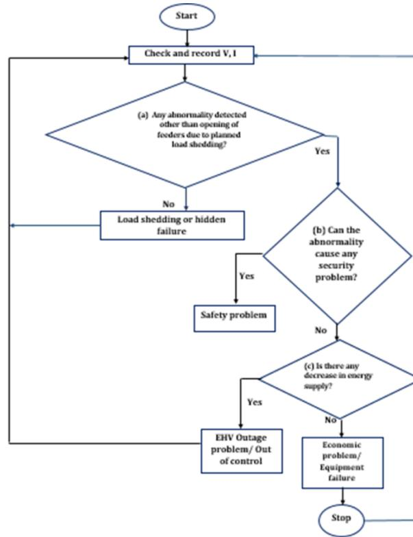
Figure 9: Flow chart for monitoring and fault detection stage
