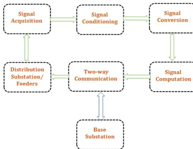
Figure 1b: Functional Block Diagram of the Smart Monitoring and Fault Detection System
