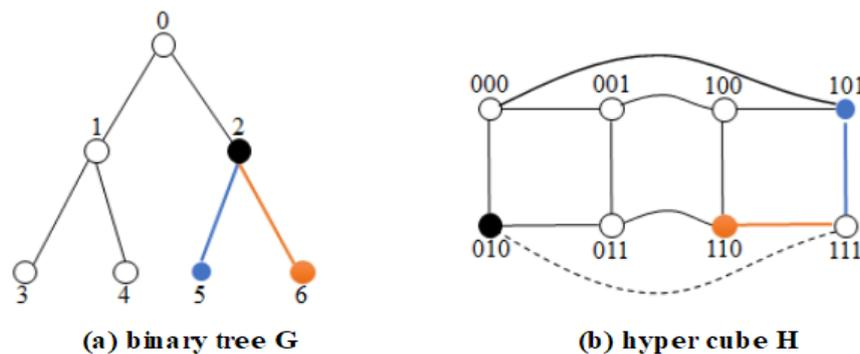
Figure 2. Embedding binary tree into hypercube Q3
