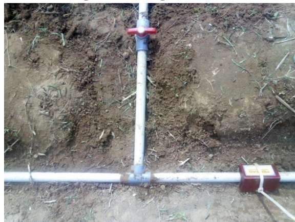
Plate 4. Magnetic fluid conditioner attached to control line
