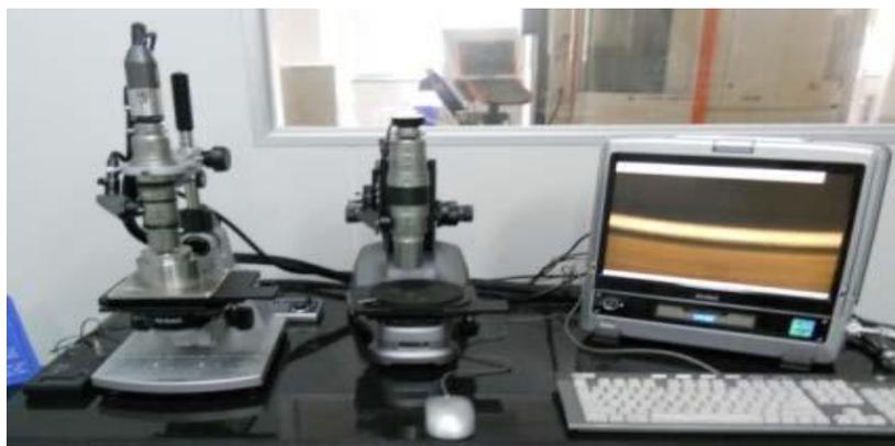
**Figure 3: The chip imaging system's microscopic vision system (see online version for colours)**
