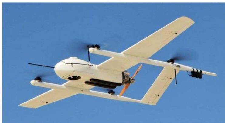
Figure 4: Fixed Wing hybrid VTOL UAV
