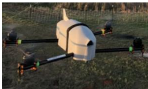
Figure 2: CopterSonde (Fixed Wing) UAV
