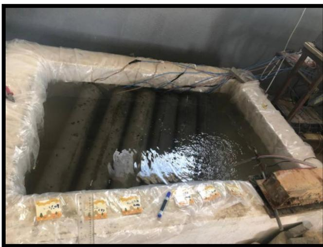
a) the corrosion cell during operation
