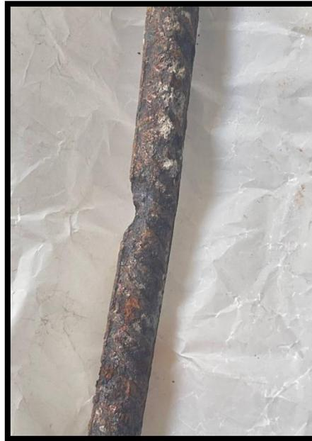
**Fig.10:Corroded Steel Bar**
