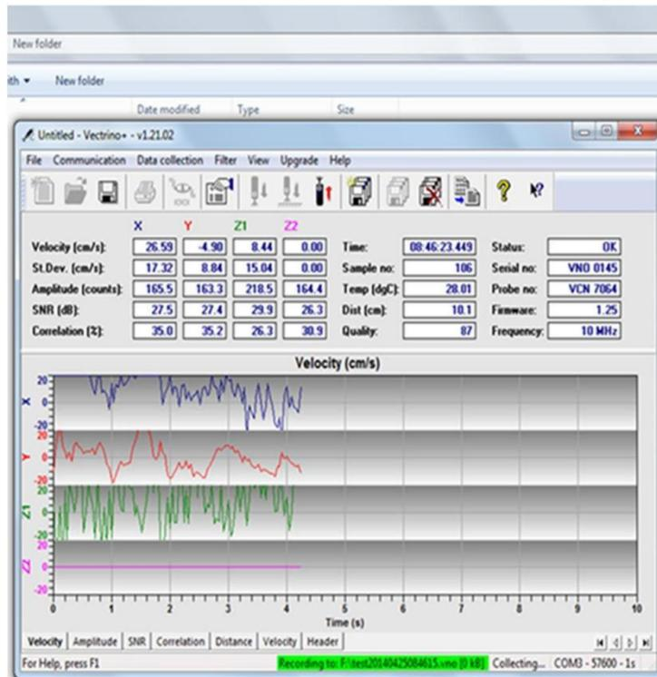
Figure 2. Velocity reading recorded in Vectrino plus software
