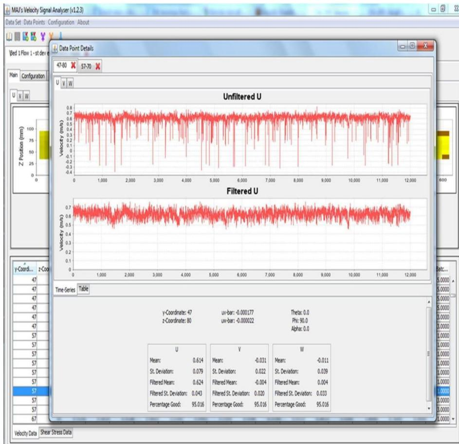
Figure 3 Velocity Signal Analyzer software (De-spiking velocity readings)
