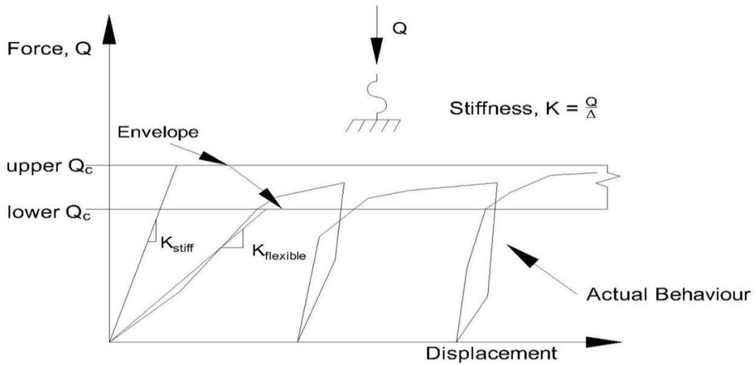
Basic Force-Displacement Envelope for Soils Components
