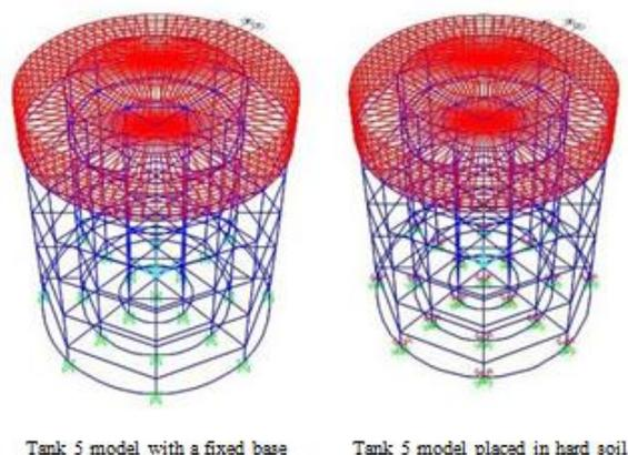
Figure 5 Model of tank 5 with a fixed base and hard soil stiffnesses
