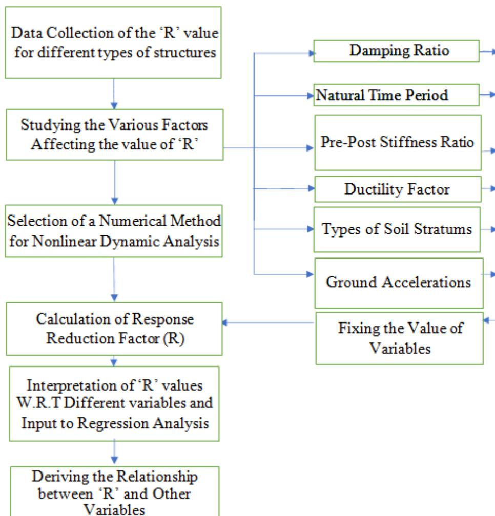
**Figure 2.** Procedure in arriving response reduction factor for overhead water tanks
