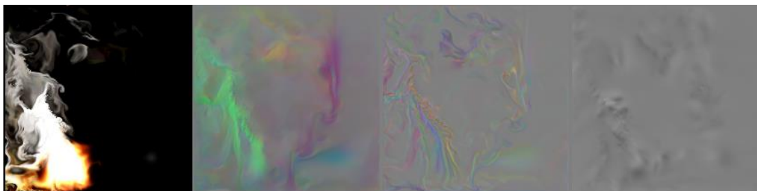
Figure 7. The individual status fields of the fluid saved in textures. Excerpts of textures from left to right: particle field, velocity field (gray is no speed, green is speed in positive y-direction, purple in negative y-direction), vorticity conservation, Pressure field (gray is no pressure, white is high pressure and black is lower pressure).
