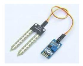
The voltage that the sensor outputs changes accordingly to the water content in the soil.
