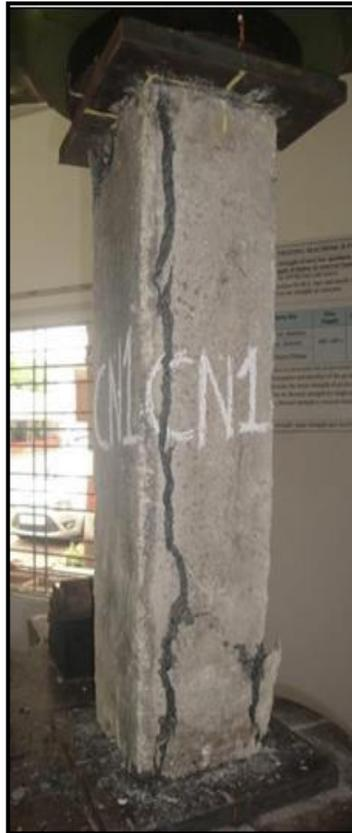
**Figure3.7.4: Nano Silica Retrofitted Column Specimen Failure at Ultimate Load**
