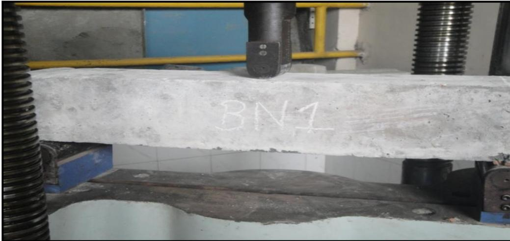
**Fig.3.3.1: Simply supported beam testing**
