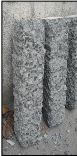
**Figure 3.5.4: Cutting of Damaged Portion of Column Specimen for Retrofitting**
