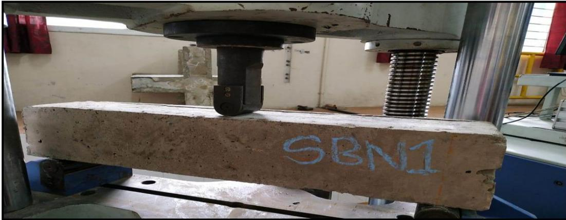
**Fig.3.4.1: Beam specimen for testing**
