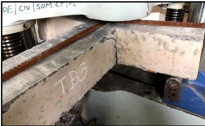
**Figure3.7.2: Nano Silica Retrofitted T-Beam Specimen Failure at Ultimate Load**
