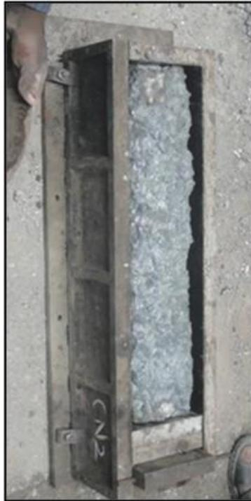
**Figure3.6.4: Moulding of column Specimens before Nano Silica Retrofitting**
