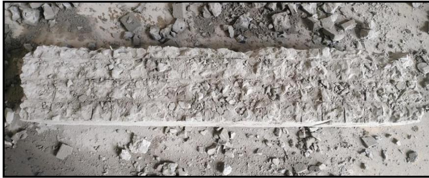
**Figure3.5.1: Cutting of Damaged Portion of Simple Beam Specimen for Retrofitting**
