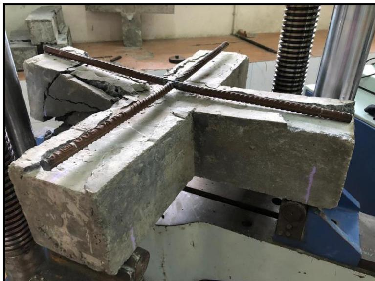
**Figure3.7.3: Nano Silica Retrofitted Cross Beam Specimen Failure at Ultimate Load**
