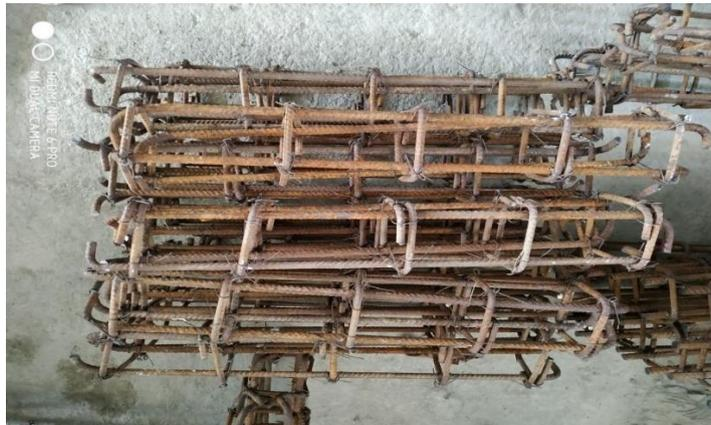
Fig. 2 Reinforcement specimen of beam
