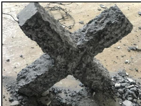
**Figure3.5.3: Cutting of Damaged Portion of Cross Beam Specimen for Retrofitting**
