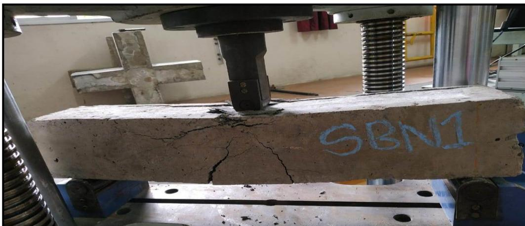
**Fig.3.4.2: Failure retrofitted beam using nano silica**
