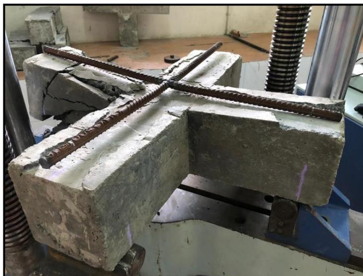
**Figure3.6.3: Testing of Nano Silica Retrofitted Cross Beam Specimen**
