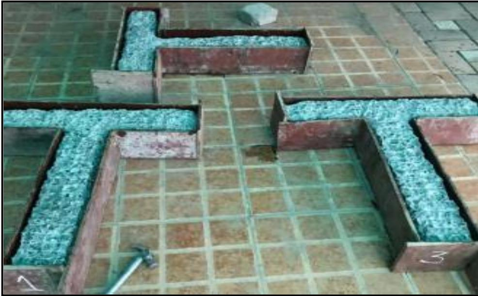
**Figure3.6.2: Moulding of T-Beam Specimens before Nano Silica Retrofitting**
