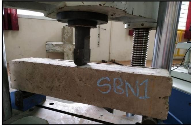
**Figure3.6.1: Testing of Nano Silica Retrofitted Beam Specimen**
