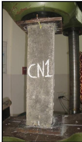
**Figure 3.6.4: Testing of Nano Silica Retrofitted Column Specimen**
