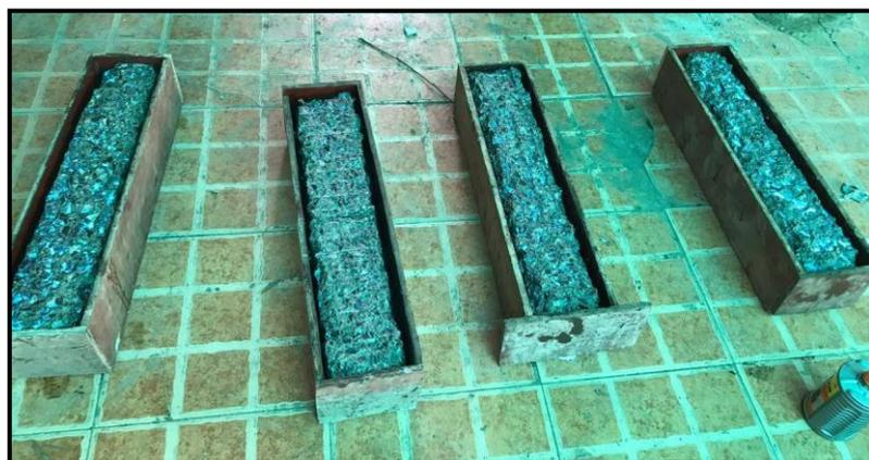
**Figure 3.6.1: Moulding of Simple Beam Specimens before Nano Silica Retrofitting**
