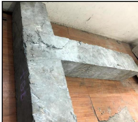
**Figure3.6.2: Testing of Nano Silica Retrofitted T-Beam Specimen**
