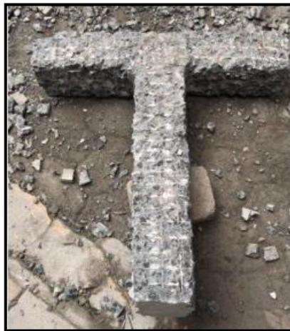
**Figure3.5.2: Cutting of Damaged Portion of T-Beam Specimen for Retrofitting**
