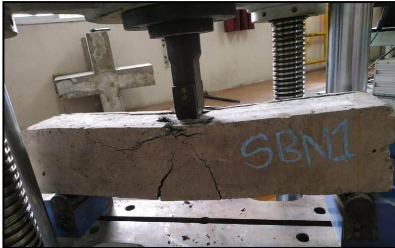
**Figure3.7.1: Nano Silica Retrofitted Simple Beam Specimen Failure at Ultimate Load**
