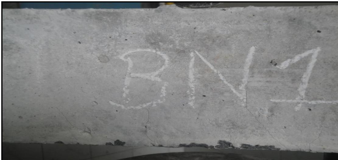
**Fig.3.3.2: First crack on beam**
