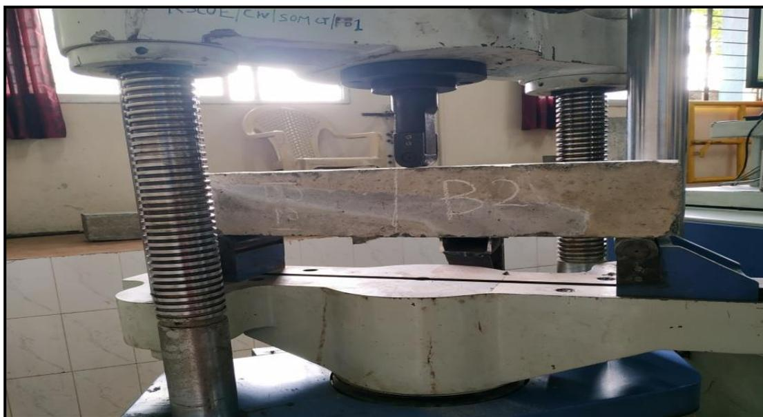
**Fig.3.2.1: Beam specimen for testing**
