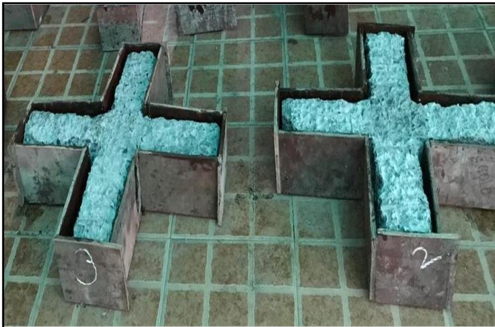
**Figure3.6.3: Moulding of Cross Beam Specimens before Nano Silica Retrofitting**
