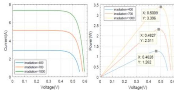
Figure 6: I-V and P-V characteristics of Single cell PV model using Sim Electronics Simulation Model
