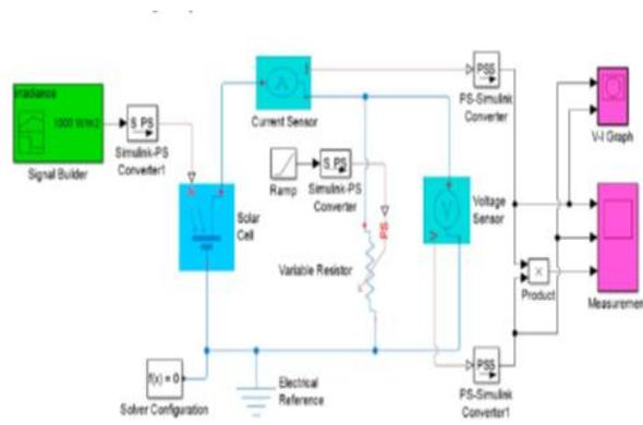
Figure 5: Simulation Model for a single Cell
