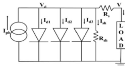
Figure 4: Practical triple diode model for PV cell.
