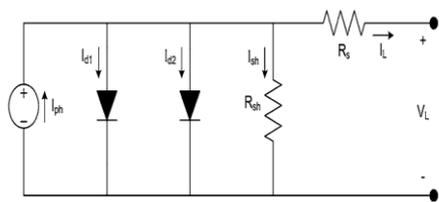
Figure 3: Practical Double diode model for PV cell.
