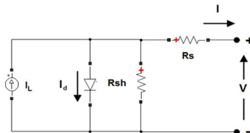
Figure 2 Practical one diode model for solar cell.
