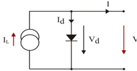
Figure 1 One diode model for PV cell.
