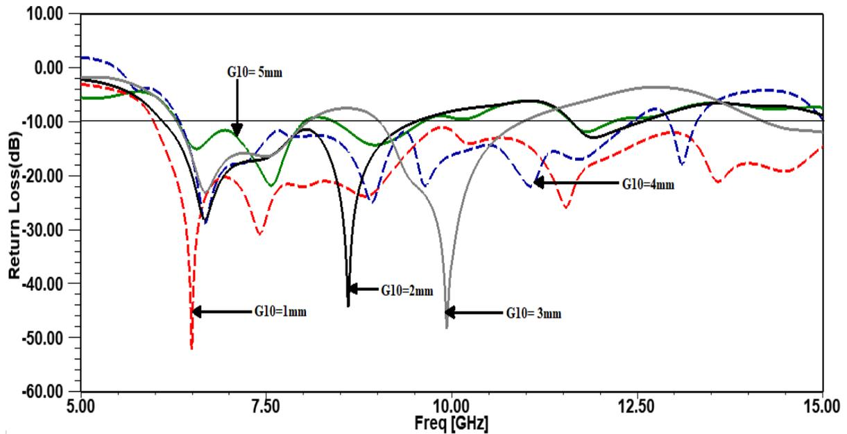
fig10. Presence of gap in the return loss
