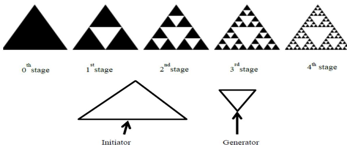
Fig. 1 different stages of fractal antenna
