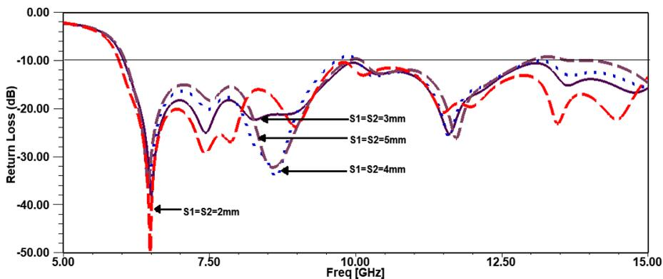
fig 9. return loss due to the presence of two split rings
