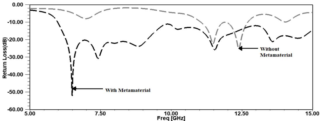
fig 8 return losses with and without the metamaterial
