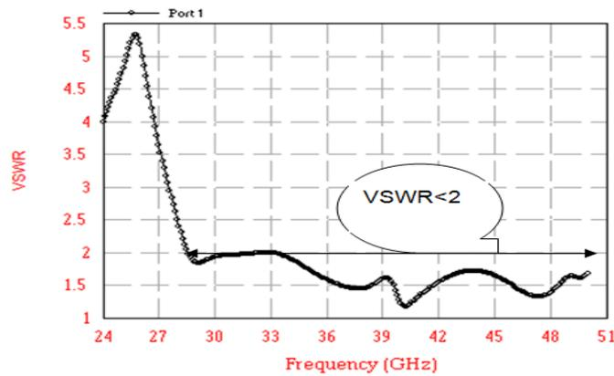
**Fig 3 Simulated Results for VSWR versus frequency plot of the proposed antenna**
