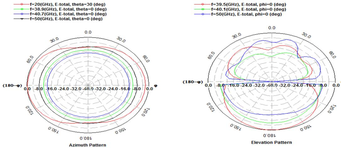
**Fig 9 Simulated Results for azimuth and elevation pattern of the proposed antenna**
