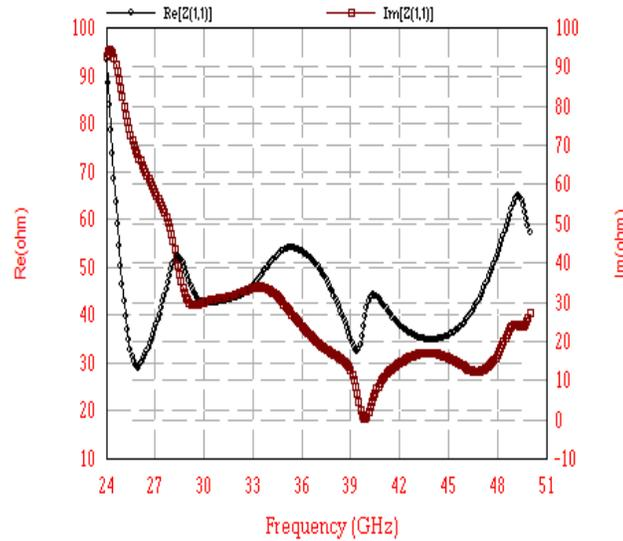
**Fig 5 simulates Results for real and imaginary resistance of the proposed antenna**
