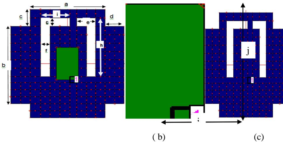
**Fig 1. Design of the proposed antenna (a) Top view of (b) Radiating Patch, (c) Ground Plane**
