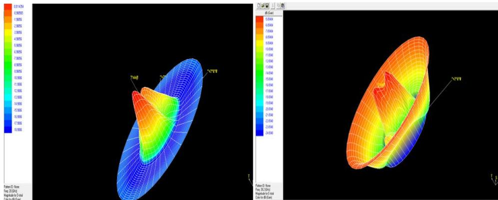
**Fig 10 3D view of Radiation Pattern of an antenna**
