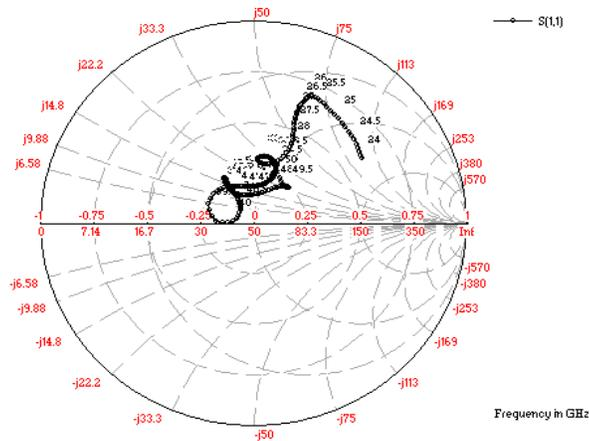
**Fig 4 Simulated Results for Switch Chart of the proposed antenna**
