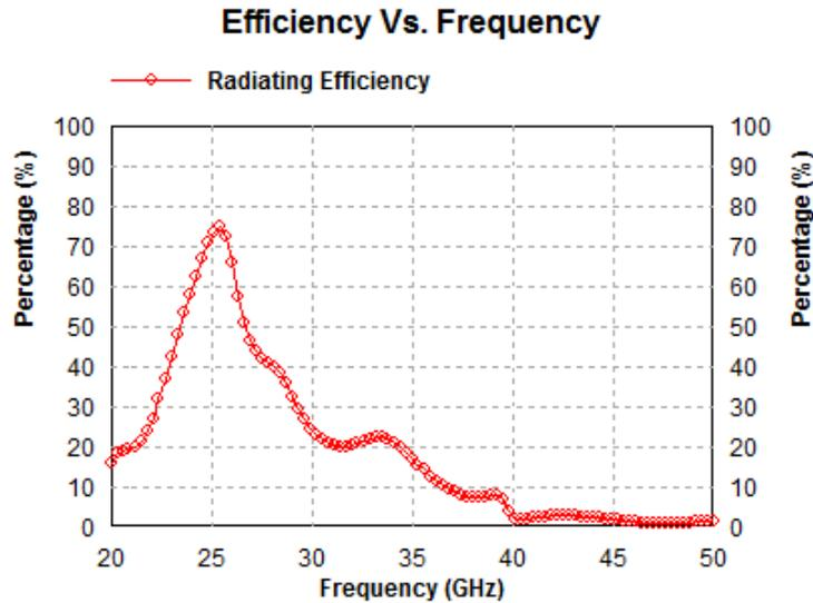
**Fig 8 Radiation efficiency and antenna efficiency of the proposed antenna with respect to frequency**
