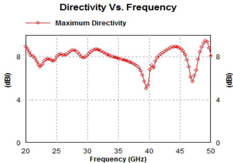
**Fig 6 Simulated Results for Directivity of the proposed antenna**
