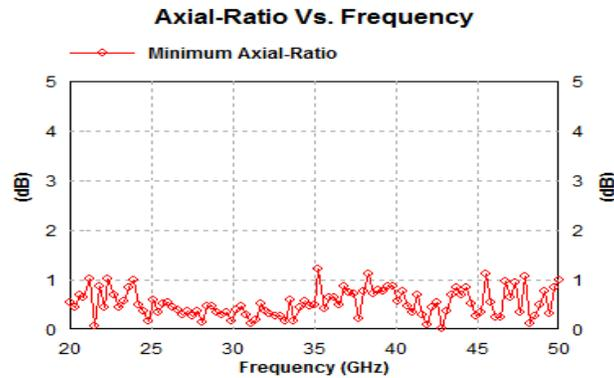
**Fig 7 Simulated Results for axial ratio of the proposed antenna**
