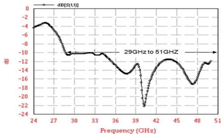
**Fig2 Simulated Reflection Coefficient versus frequency plot of the proposed antenna**
