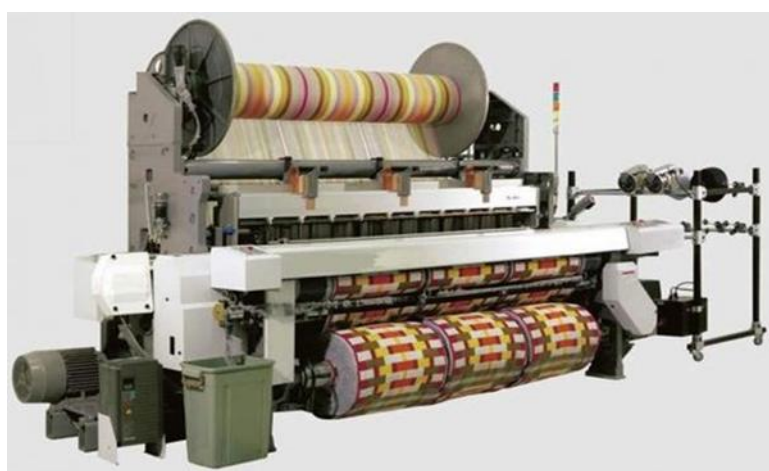
Fig-1 Textile rapier weaving loom
