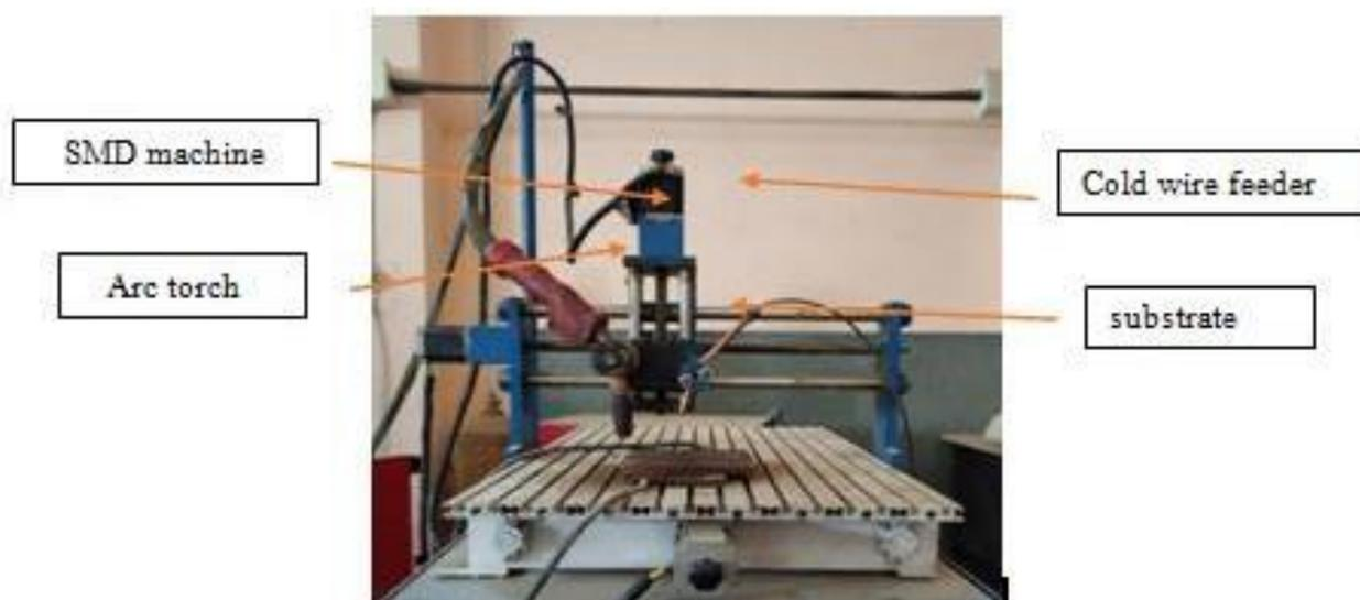
**Figure (1) Close-up view of the deposition unit.**
