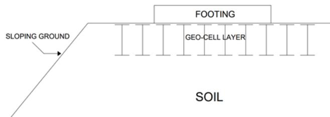
**Fig. 1.** Schematic Representation
