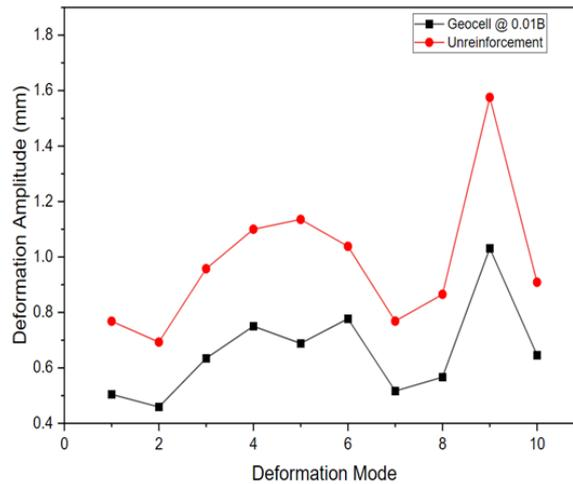
**Fig. 8.** Displacement variation in unreinforced case
