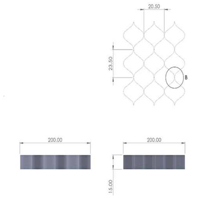
**Fig. 3.** Geocell modelled in the analysis (dimensions are in mm).
