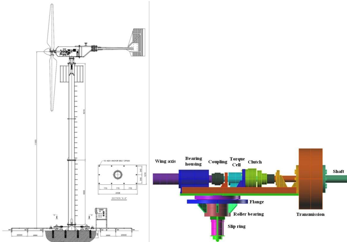
**Fig. 2; A Sketch of Seawater Exchange System with Wind Power**
