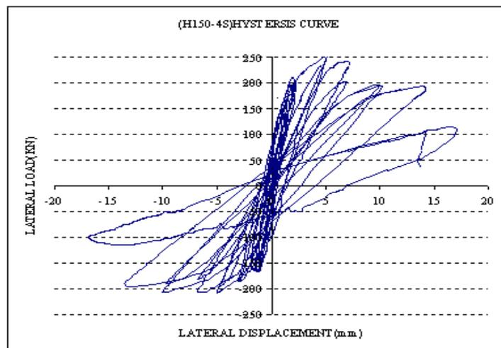
Figure 23; Reinforced Masonry Wall Hysteresis Diagram (H150-4s)
