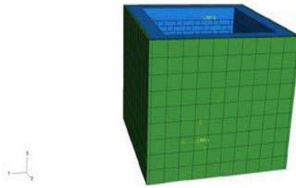
Figure 9; Un-deformed Model of the Reinforced Specimen
