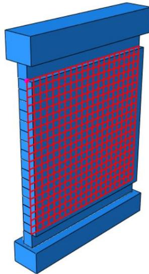
**Figure 15; Connection of Shotcrete Concrete and a Rebars Mesh inside the Concrete**
