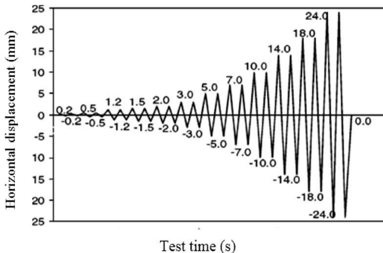
**Figure 2; Lateral Loading Method in Cyclic Shear Test [11]**
