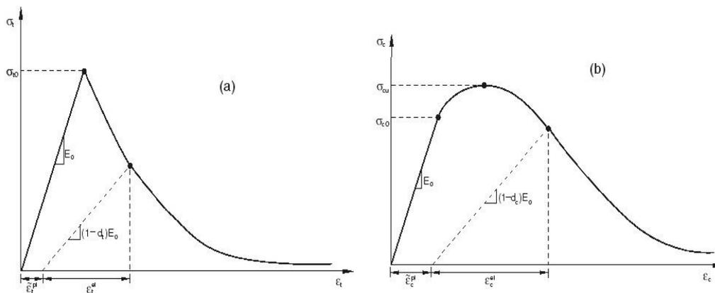
**Figure 5; Response of Concrete to Uniaxial Loading in Tensile (a) and High Pressure (b) [12]**
