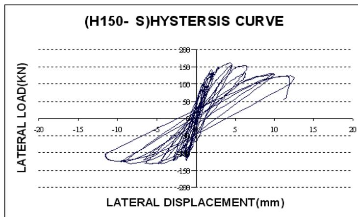
Figure 22; Diagram of Reinforced Masonry Wall Hysteresis (H150-2s)
