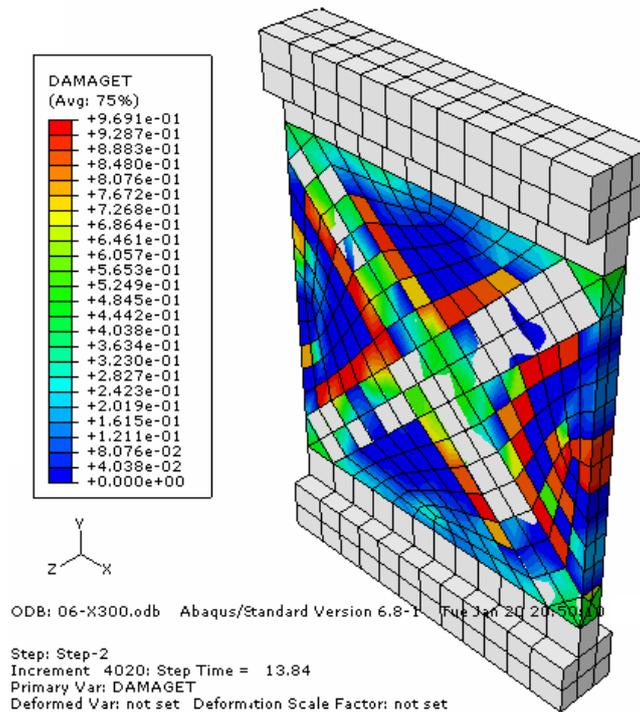
**Figure 28; Strain- stress Distribution Plate in Masonry Wall (X-300)**
