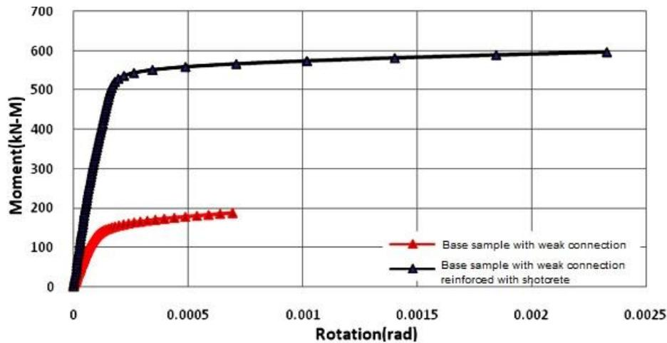
**Figure 13; Effect of Shotcrete Reinforcement on the Torsional Behavior of a Brick Building with Wall-to-wall Vulnerability**
