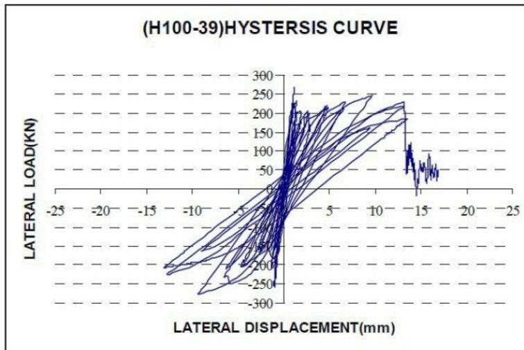
Figure 18; Diagram of Reinforced Masonry Wall Hysteresis (H100-39)
