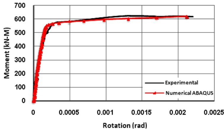
**Figure 11; Torsion Anchor-rotation Diagrams in Numerical and Laboratory Modes for Reinforced Specimen**
