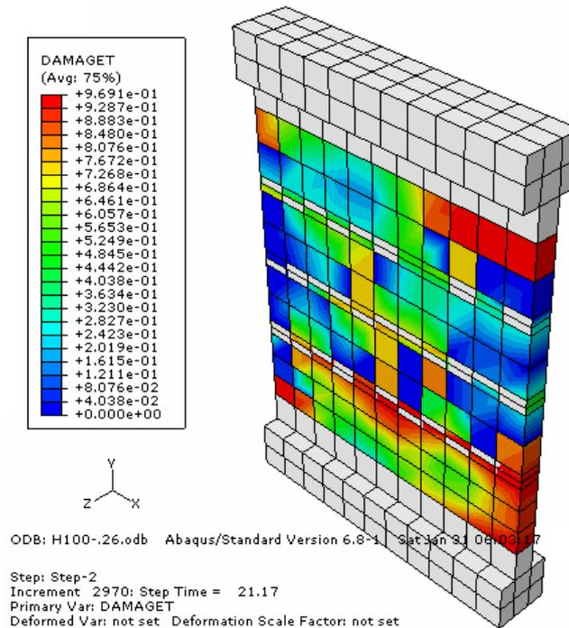
**Figure 24; Strain- stress Distribution Plane in Masonry Wall (H100-26)**
