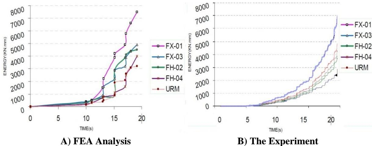
**Figure 6; Comparison between Energy-time Curves of Masonry Walls**
