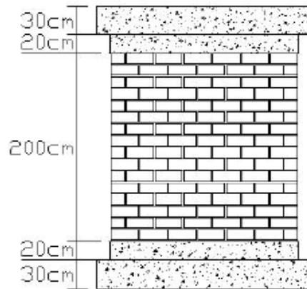
**Figure 1; Dimensions of the Wall [11]**
