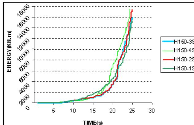
**Figure 26; Effect of the Number of FRP Strips on the Energy-time Curve**
