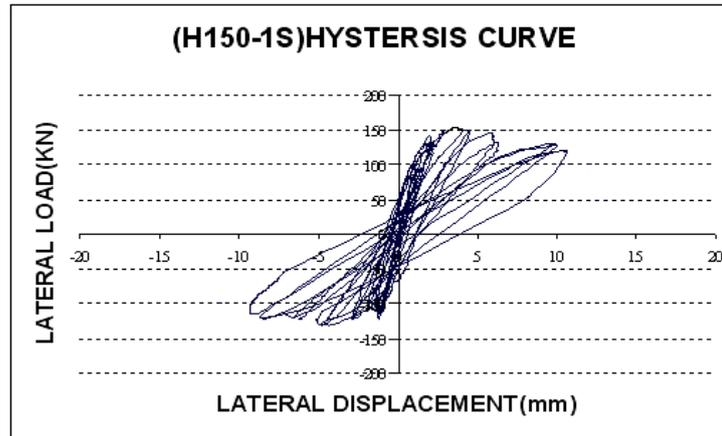
Figure 21; Diagram of Reinforced Masonry Wall Hysteresis (H150-1s)
