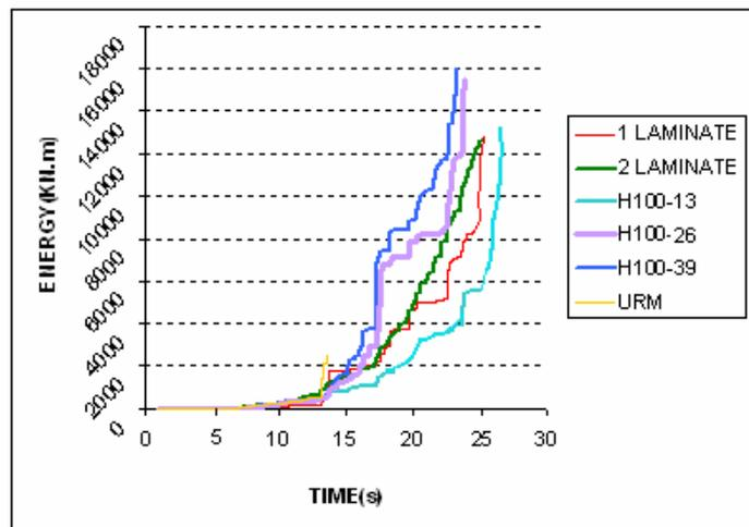
Figure 27; The Effect of FRP Layer Thickness on the Energy-time Curve
