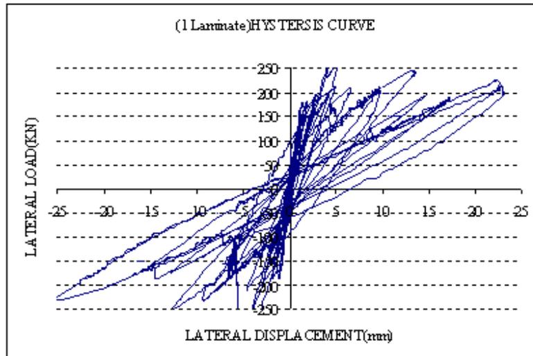
**Figure 19; Diagram of Hysteria of Reinforced Masonry Wall (1 Laminate)**
