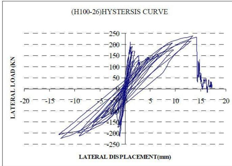
Figure 17; Reinforced Masonry wall Hysteresis Diagram (H100-26)
