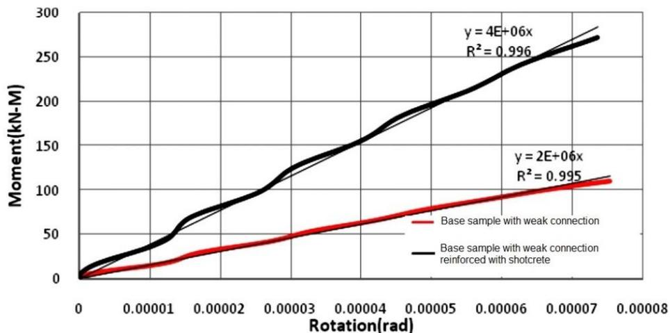
**Figure 14. Torsional Stiffness of the base Sample with Weak and Reinforced Connection**
