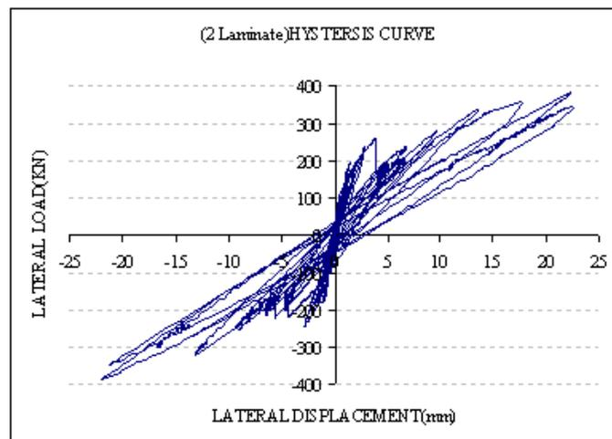
**Figure 20; Hysteria Diagram of Reinforced Masonry Wall (2 Laminates)**
