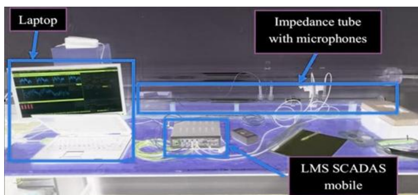
Figure 9: Apparatus set up for the estimation of sound transmission misfortune
