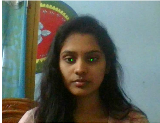
Fig. 2. Pupil detection image (green color circles indicate the detected pupil).
