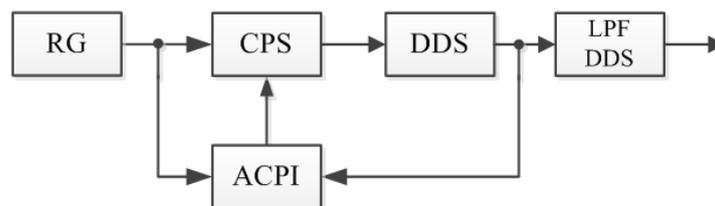
Figure 2 - A block diagram of a DDS with ACPI and deviation control
