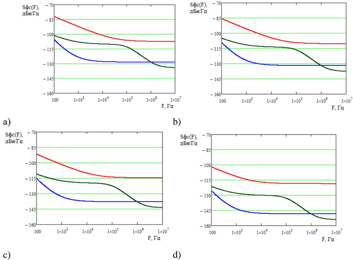
Figure 4 – Noise contributions of the components in dBc/Hz as a function of frequency offset  $F$  in Hz at 900 kHz and  $K_{DDS} = 0.3$  (a), 600 kHz and  $K_{DDS} = 0.2$  (b), 300 kHz and  $K_{DDS} = 0.1$  (c), 90 kHz and  $K_{DDS} = 0.03$  (d)
