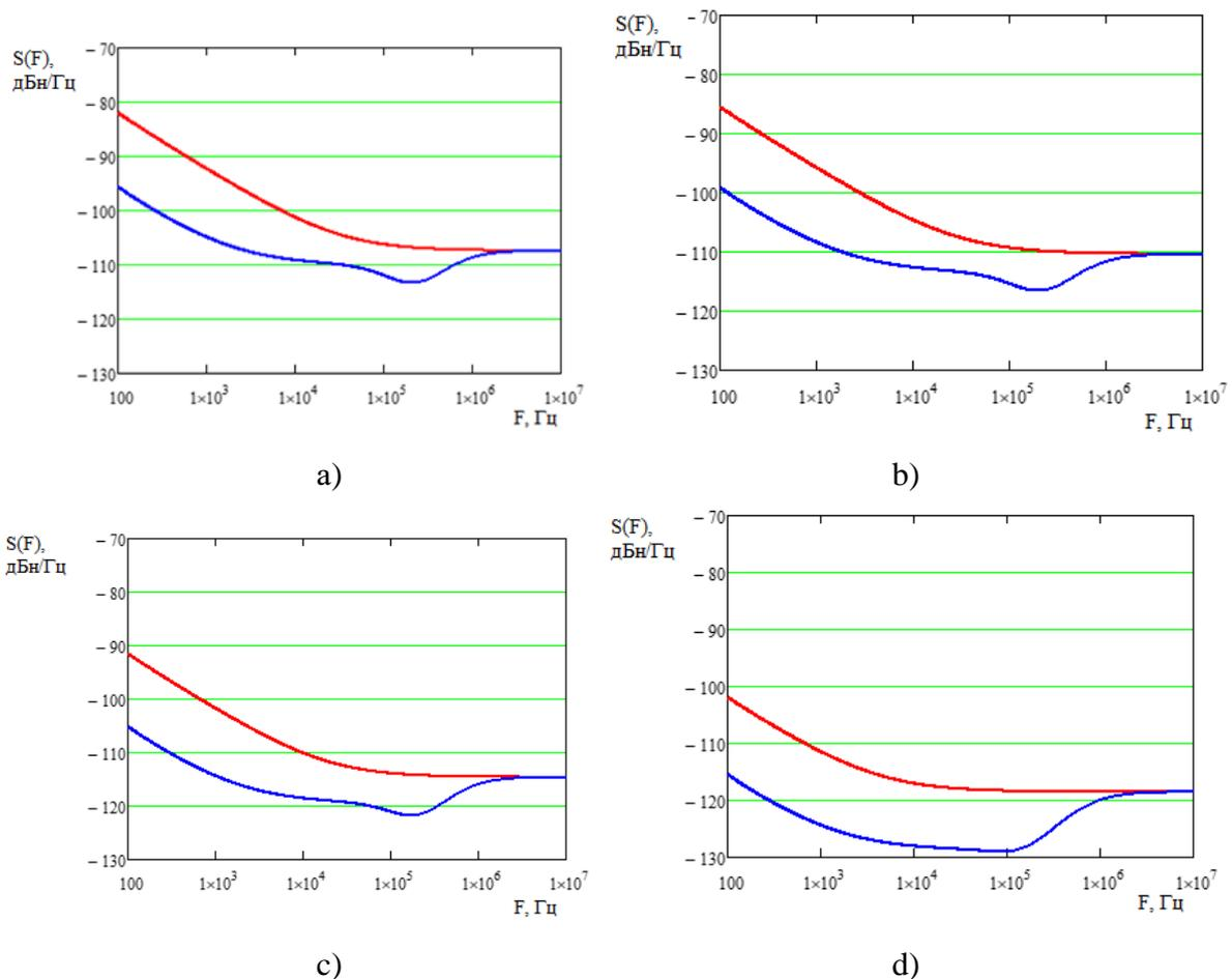
Figure 3 – SPD of the phase noise of the sounding signal generator in dBc/Hz as a function of frequency offset  $F$  in Hz at 900 kHz and  $K_{DDS} = 0.3$  (a), 600 kHz and  $K_{DDS} = 0.2$  (b), 300 kHz and  $K_{DDS} = 0.1$  (c), 90 kHz and  $K_{DDS} = 0.03$  (d)
