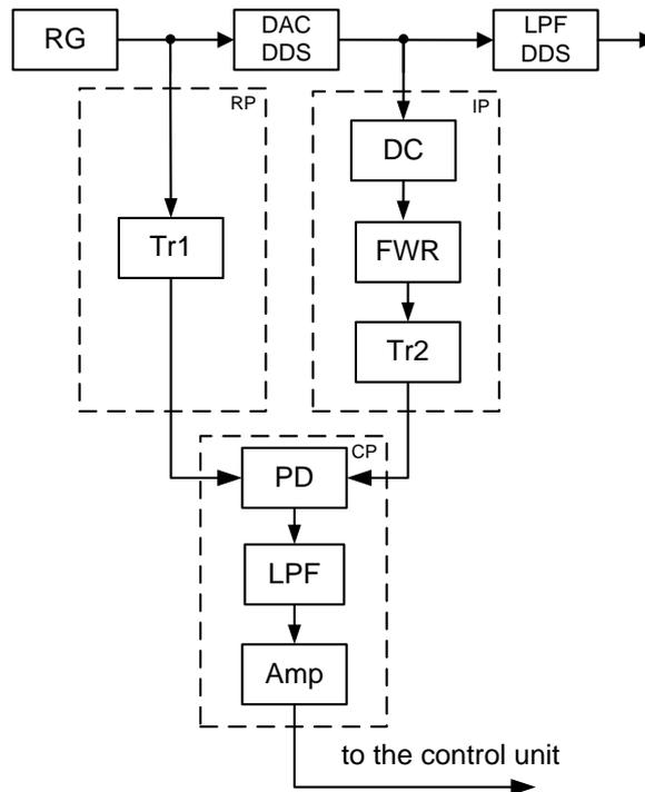
Fig. 1 - Block diagram of the ACPI control signal formation path
